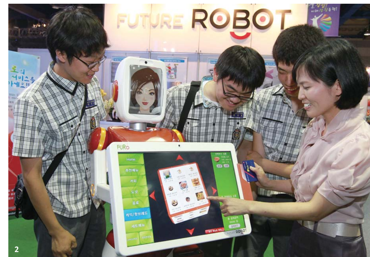
2. FURo (Future Robot), an intelligent service robot that can display human-like emotions while taking orders or providing information.
